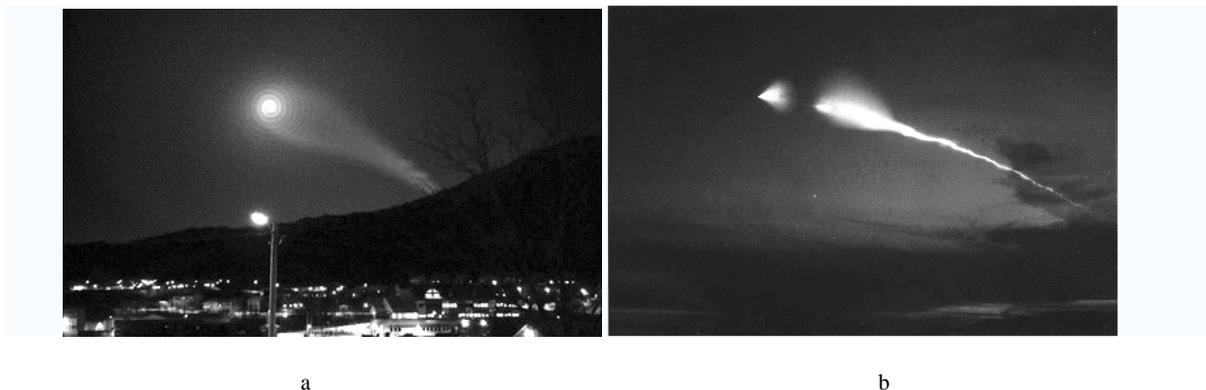
Fig. 1. Rocket track visible as a result of the scattering of sunlight on the products of combustion. During a) the White Sea launch b) during the Vandenberg launch
